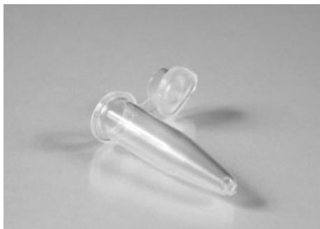
Figure 1. Standard 0.5-ml microcentrifuge vial with plastic cap used for TIBS. Thrips are collected through a hole at the narrow end of the vial. The well of the cap is filled with a sugar-water solution and sealed with parafilm.
