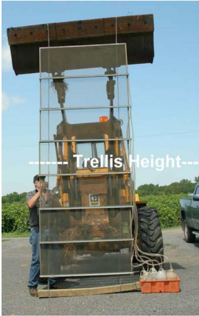
**NY grape grower, patternator stored in the barn, note screens attached to chains so can be mounted on a fork lift or tractor fore-loader**
